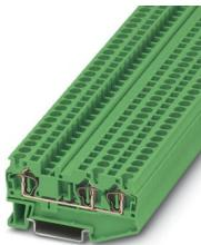
Feed-through terminal block, nom. voltage: 800 V, nominal current: 32 A, number of connections: 3, connection method: Spring-cage connection, Rated cross section: 4 mm<sup>2</sup>, 1 level, cross section: 0.08 mm<sup>2</sup> - 6 mm<sup>2</sup>, mounting type: NS 35/7,5, NS 35/15, color: green
