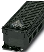
Fuse modular terminal block, fuse type: Glass / ceramics / ..., fuse type: G / 5 x 20 / 5 x 25 / 5 x 30, nom. voltage: 24 V, nominal current: 6.3 A, number of positions: 1, connection method: Screw connection, Rated cross section: 4 mm<sup>2</sup>, cross section: 0.2 mm<sup>2</sup> - 4 mm<sup>2</sup>, mounting type: NS 35/7,5, NS 35/15, NS 32, color: black
