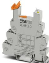
14 mm PLC basic terminal block with screw connection, without relay or solid-state relay, for mounting on DIN rail NS 35/7,5, 2 changeover contacts, input voltage 24 V AC/DC
