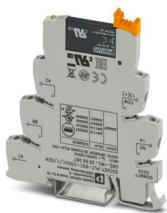
PLC-INTERFACE for input functions, consisting of PLC-BSC.../SEN basic terminal block with screw connection and plug-in miniature solid-state relay, for mounting on DIN rail NS 35/7,5, 1 N/O contact, input: 230 V AC/220 V DC, output: 3 - 48 V DC/100 mA
