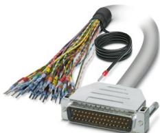
Assembled shielded round cable; connection 1: Single wires (50-position) (The wires are marked and fitted with ferrules. The braided shield is routed to a separate cable end.); connection 2: D-SUB pin strip (1x 50-position); cable length: 4 m
