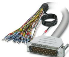
Assembled shielded round cable; connection 1: Single wires (50-position) (The wires are marked and fitted with ferrules. The braided shield is routed to a separate cable end.); connection 2: D-SUB pin strip (1x 50-position); cable length: 1 m
