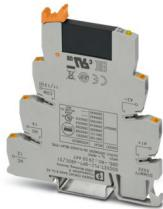
PLC-INTERFACE, consisting of PLC-BPT.../21 basic terminal block with push-in connection and plug-in miniature solid-state relay, for mounting on DIN rail NS 35/7,5, 1 N/O contact, input: 48 V DC, output: 3 - 48 V DC/100 mA
