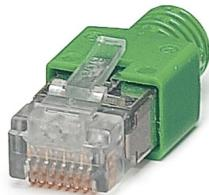
RJ45 connector, design: RJ45, degree of protection: IP20, number of positions: 8, 1 Gbps, CAT5 (IEC 11801:2002), material: Plastic, connection method: Crimp connection, connection cross section: AWG 26- 24, cable outlet: straight, color: gray, Ethernet
