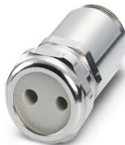
Accessories for FL-WLAN 1100 series: Optional cable feed-through for sealing (IP67) the FL-WLAN 110x connection (IP20), if the device is not directly integrated onto the closed housing. Not needed when mounting on a control cabinet, etc.
