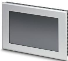
Panel PC, 17.8 cm / 7"-TFT display (analog resistive (polyester)), 800 x 480 pixel(s) (WVGA), 262144 colors, AMD® Embedded G-Series (T40E), 2x 1 GHz, 4x USB Host 2.0, 2x Ethernet (10/100/1000 Mbps), RJ45, Windows® Embedded Standard 7, Movicon™, without bus system.
