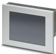
Touch panel, 14.5 cm / 5.7"-TFT display (analog resistive (polyester)), 320 x 240 pixel(s) (QVGA), 65536 colors, Arm9™, 200 MHz, 2x USB Host 2.0, 1 x Ethernet (10/100 Mbps), RJ45, Windows® CE 5.0, TSvisRT, without bus system.
