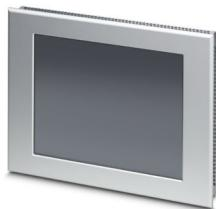
Touch panel, 26.4 cm / 10.4"-TFT display (analog resistive (polyester)), 800 x 600 pixel(s) (SVGA), 262144 colors, Xscale® PXA320, 806 MHz, 2x USB host 1.1, 1 x Ethernet (10/100 Mbps), RJ45, Windows® CE 6.0, Movicon™, without bus system.
