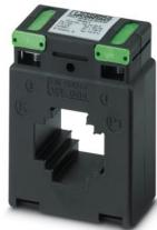
Window-type current transformer, 75 A AC primary current; 5 A AC secondary current; accuracy class 1; 1.5 VA rated power
