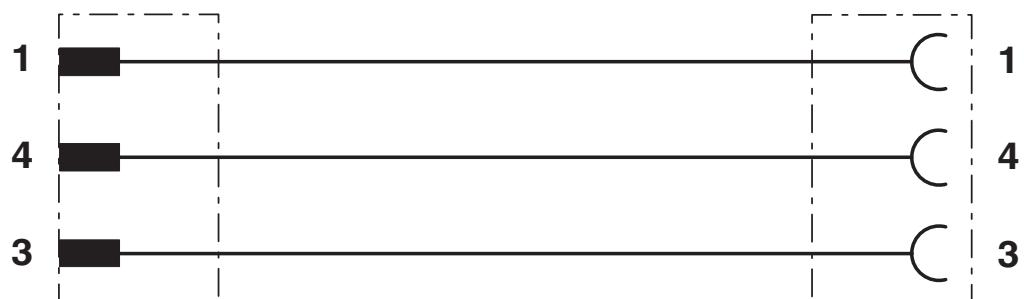
Contact assignment of M12 plugs / M8 sockets
