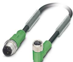
Sensor/actuator cable, 3-position, PUR halogen-free, black-gray RAL 7021, Plug straight M12, coding: A, on Socket angled M8, coding: A, cable length: 1.5 m
