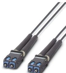
Assembled FO cable, breakout cable, 980/1000 µm polymer fiber, SC-RJ/IP20 to SC-RJ/IP20, for installation inside control cabinets, the cable is suitable for UV-protected outdoor use, length: 1 m
