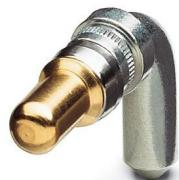
POWER contact, for D-SUB combination inserts, for PCB assembly, pin, angled, rated current 40 A, gold-plated
