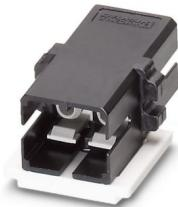
SC-RJ coupling insert, duplex, for VS-PP-19-1HE-16-F patch panel, VS-TO...F... terminal outlets, and VS-SI-FP-2F front plate, can be used for GOF (multi-mode and single mode), HCS, and polymer fiber types
