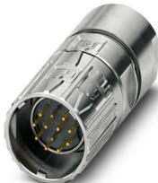
M23, Cable connector, series: M23 PRO, straight, shielded: yes, ONECLICK fast locking system, No. of pos.: 12, Direction of rotation: Standard, contact connection type: Pin, Crimp connection, cable diameter range: 9 mm ... 15 mm, coding: N, Item is lead-free in accordance with RoHS II without Exemption 6c (Pb < 0.1 %)
