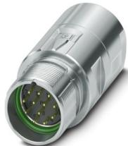
M23, Coupler connector, series: M23 PRO, straight, shielded: yes, for standard and ONECLICK fast locking system, No. of pos.: 12, Direction of rotation: Standard, contact connection type: Pin, Crimp connection, cable diameter range: 4 mm ... 8.5 mm, coding: N, Item is lead-free in accordance with RoHS II without Exemption 6c (Pb < 0.1 %)
