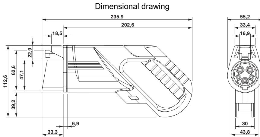
Make sure that the vehicle charging connector is placed in an appropriate charging connector holder, which ensures a minimum protection rating of IP24 in accordance with IEC 61851-1, for the entire time between charging. To create this charging connector holder, use the dimensions of the vehicle charging connector. Detailed dimensions can also be found in the Download area.
