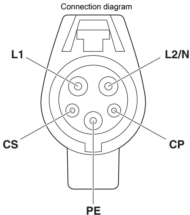
Pin assignment of the Vehicle Connector
