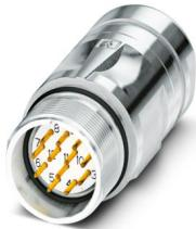
M23, Coupler connector, series: CA, straight, shielded: yes, for standard and SPEEDCON interlock, No. of pos.: 12, Direction of rotation: Standard, contact connection type: Pin, Solder cup, cable diameter range: 3 mm ... 14.5 mm, coding: N, this item is expected to be lead-free from Q1 2026 in accordance with RoHS II without exception 6c (Pb < 0.1%), a lead-free alternative is possible on request in advance
