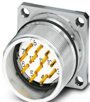
M23, Device connector front mounting, series: CA, straight, shielded: yes, for standard and SPEEDCON interlock, No. of pos.: 12, Direction of rotation: Standard, contact connection type: Pin, Crimp connection, Flat gasket, flange dimensions: 25 mm x 25 mm, coding: N
