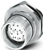
M23, Device connector rear mounting, series: CA, straight, shielded: yes, for standard and SPEEDCON interlock, No. of pos.: 16, Direction of rotation: Standard, contact connection type: Socket, Crimp connection, Axial seal, coding: N, this item is expected to be lead-free from Q1 2027 in accordance with RoHS II without exception 6c (Pb < 0.1%), a lead-free alternative is possible on request in advance
