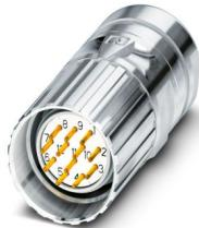
M23, Cable connector, series: CA, straight, shielded: yes, Screw locking mechanism, No. of pos.: 17, Direction of rotation: Standard, contact connection type: Pin, Solder connection, cable diameter range: 3 mm ... 14.5 mm, coding: N, this item is expected to be lead-free from Q2 2026 in accordance with RoHS II without exception 6c (Pb < 0.1%), a lead-free alternative is possible on request in advance
