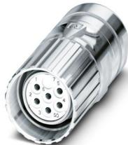
M23, Cable connector, series: CA, straight, shielded: yes, Screw locking mechanism, No. of pos.: 8+1, Direction of rotation: Standard, contact connection type: Socket, Crimp connection, cable diameter range: 6 mm ... 10 mm, coding: N, this item is expected to be lead-free from Q2 2026 in accordance with RoHS II without exception 6c (Pb < 0.1%), a lead-free alternative is possible on request in advance
