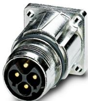
Device connector front mounting, straight, for standard and SPEEDCON interlock, M17, number of positions: 6+PE, contact connection type: Pin, shielded: yes, flange dimensions: 21.6 mm x 21.6 mm, number of positions: 7, connection method: Crimp connection, series: ST
