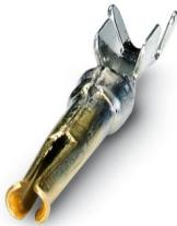
Crimp contact, Socket, rolled, contact diameter: 1 mm, connection cross section: 0.22 mm<sup>2</sup> ... 0.56 mm<sup>2</sup>, contact material: Cu alloy, Item is lead-free in accordance with RoHS II without Exemption 6c (Pb < 0.1 %)
