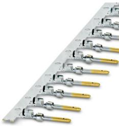
Crimp contact, Pin, rolled, contact diameter: 1 mm, connection cross section: 0.22 mm<sup>2</sup> ... 0.56 mm<sup>2</sup>, contact material: Cu alloy, Taped product, 10000 Pcs. per ribbon, Item is lead-free in accordance with RoHS II without Exemption 6c (Pb < 0.1 %)
