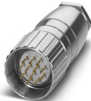
M23, Cable connector, series: RC, straight, shielded: no, Screw locking mechanism, No. of pos.: 16, Direction of rotation: Standard, contact connection type: Pin, Solder cup, coding: N, this item is expected to be lead-free from Q4 2025 in accordance with RoHS II without exception 6c (Pb < 0.1%), a lead-free alternative is possible on request in advance
