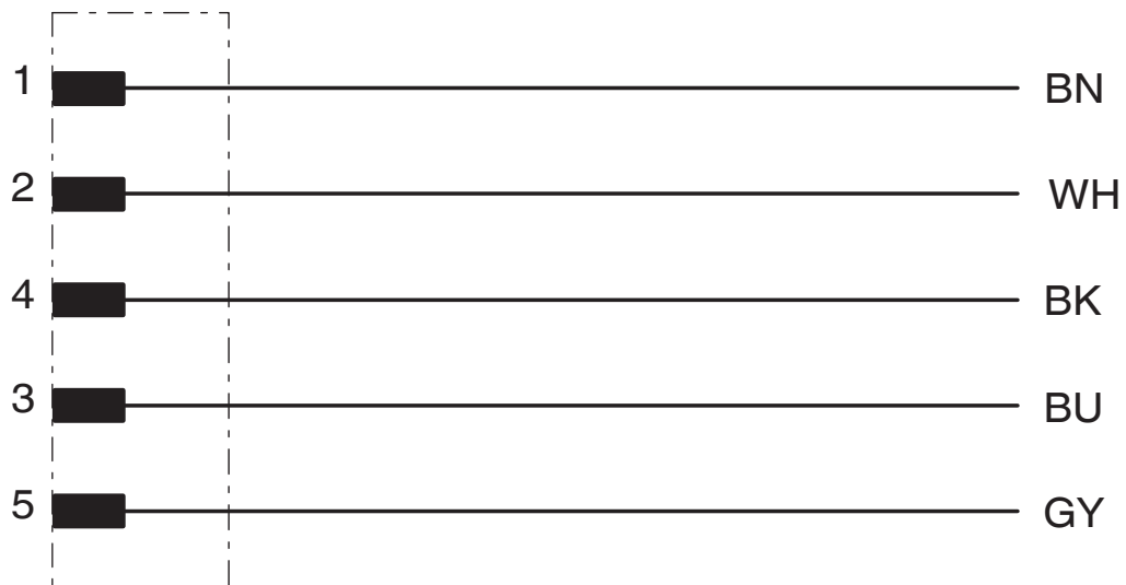
Contact assignment of the M12 plug
