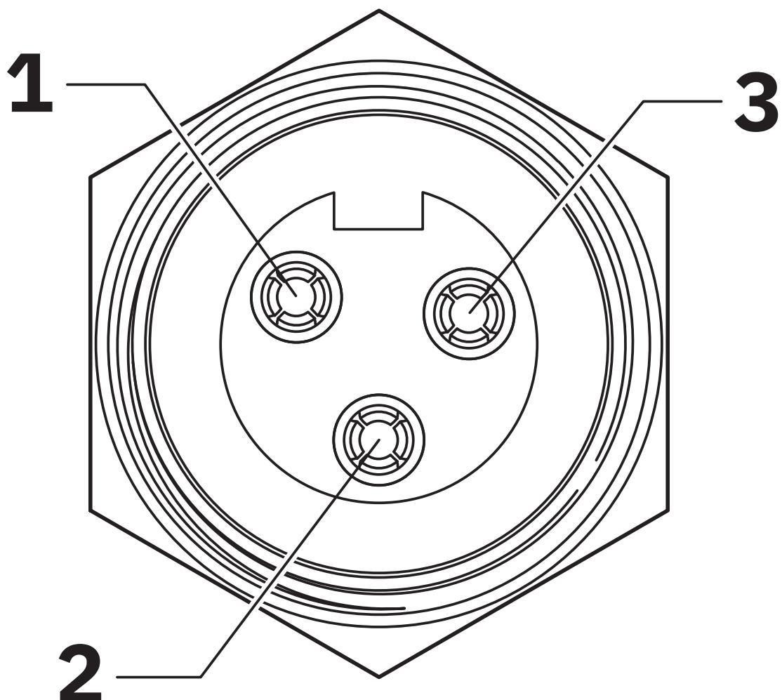
Pin assignment, socket, 1-3/8"-16UN, 3-pos., view of female side
