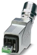
RJ45 connector, degree of protection: IP65/IP67, number of positions: 8, 1 Gbps, CAT5, material: Metal, connection method: IDC fast connection, connection cross section: AWG 23- 22, cable outlet: angled, Ethernet
