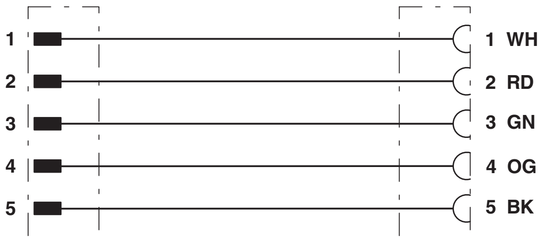
Contact assignment of 7/8" plugs/sockets
