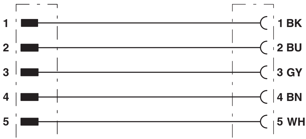
Contact assignment of 7/8" plugs/sockets
