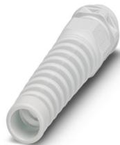
Cable gland, material for screw connection: PA, application: Standard, external cable diameter 9 mm ... 17 mm, shielding: no, connecting thread: M25 x 1.5, color: lightgray RAL 7035, with bend protection sleeve
