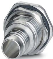
Housing screw connection, Pin, M8-Screw locking mechanism, this item is expected to be lead-free from Q2 2026 in accordance with RoHS II without exception 6c (Pb < 0.1%), a lead-free alternative is possible on request in advance
