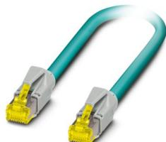
Patch cable, CAT6<sub>A</sub>, 4-pair, shielded, connection not crossed (line), assembled at both ends with RJ45/IP20 connectors, outer sheath material: PUR, length: 6.0 m
