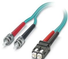
Assembled FO cable, zip cord cable, multi-mode fiberglass 50/125 µm, OM3, plug: B-FOC (ST)/SC-RJ, degree of protection: IP20, for installation in cable ducts or control cabinets, length: 2 m
