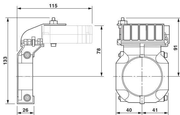
Fan for horizontal attachment to the panel feed-through
