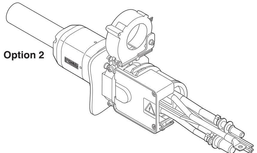
Select one option for mounting the fan. Illustrated using straight panel feed-through as an example.
