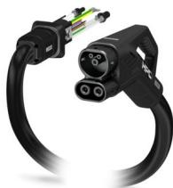
CHARX connect professional, CCS type 2, HPC DC charging cable, up to 700 A in Boost mode, 500 A permanent, 1000 V DC, with cooled vehicle charging connector and cooled cable, cable: 3 m, black, straight, with replaceable mating face frame, with replaceable DC power contacts, with straight panel feed-through, with variable-speed fan, PHOENIX CONTACT logo, IEC 62196-3-1, for charging electric vehicles (EV) with direct current (DC)
