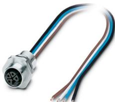
Device connector front mounting, Power, 4-position, Flush-type female connector, straight, M12-Standard, L-coding, on free cable end, Individual wires, cable length: 0.5 m, 2.50 mm<sup>2</sup>, PEX litz wire
