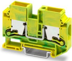
Protective conductor terminal block, number of connections: 2, number of positions: 1, connection method: Push-X-connection, Rated cross section: 16 mm<sup>2</sup>, cross section: 2.5 mm<sup>2</sup> - 25 mm<sup>2</sup>, mounting type: NS 35/7,5, NS 35/15, color: green-yellow
