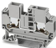
Feed-through terminal block, nom. voltage: 1000 V, nominal current: 41 A, number of connections: 2, number of positions: 1, connection method: Push-X-connection, Rated cross section: 6 mm<sup>2</sup>, cross section: 0.5 mm<sup>2</sup> - 10 mm<sup>2</sup>, mounting type: NS 35/7,5, NS 35/15, color: gray
