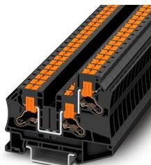
Feed-through terminal block, nom. voltage: 1000 V, nominal current: 41 A, number of connections: 3, number of positions: 1, connection method: Push-in connection, Rated cross section: 6 mm<sup>2</sup>, cross section: 0.5 mm<sup>2</sup> - 10 mm<sup>2</sup>, mounting type: NS 35/7,5, NS 35/15, color: black
