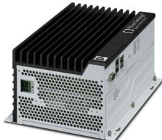
Safety controller (SPS), PLCnext Control; Programming: High-level language and IEC 61131-3; Operating system: Yocto/Linux® (real-time); Programming tool: PLCnext Engineer, Eclipse®, Visual Studio®, MATLAB®/ Simulink®; Processor: Intel® Core™ i7-10700TE, 8x 2 GHz (Standard).
