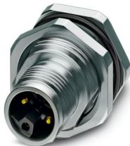
Device connector rear mounting, Power, 5-position, Pin, straight, M12, L-coding, Wave soldering, Item is lead-free in accordance with RoHS II without Exemption 6c (Pb < 0.1 %)
