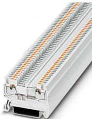
Feed-through terminal block, nom. voltage: 500 V, nominal current: 17.5 A, number of connections: 2, connection method: Push-in connection, Rated cross section: 1.5 mm<sup>2</sup>, 1 level, cross section: 0.14 mm<sup>2</sup> - 1.5 mm<sup>2</sup>, mounting type: NS 35/7,5, NS 35/15, color: white
