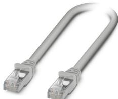
Patch cable, degree of protection: IP20, cable length: 2 m, number of positions: 8, CAT5, connection method: Pierce connection, connection cross section: AWG 26- 26, cable outlet: straight, Ethernet, 2x2xAWG26/7, S/UTP, gray
