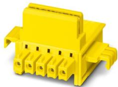
DIN rail bus connector, nominal current: 8 A (parallel contacts), rated voltage (III/2): 125 V, number of positions: 5, pitch: 3.81 mm, color: yellow, mounting: DIN rail, item with gold-plated contacts, bus connector for connecting to electronics housings, 5 parallel contacts
