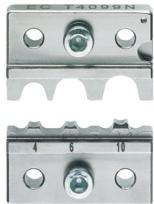
Die for CF 500 automatic crimping device, for tubular cable lugs 4 mm<sup>2</sup> ... 10 mm<sup>2</sup>, **4 mm<sup>2</sup>:** outer Ø 5 mm, inner Ø 3 mm, **6 mm<sup>2</sup>:** outer Ø 6.5 mm, inner Ø 3.5 mm, **10 mm<sup>2</sup>:** outer Ø 7 mm, inner Ø 4.5 mm
