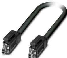
Patch cable, design: IEC 63171-2, degree of protection: IP20, cable length: 3 m, number of positions: 2, 1 Gbps, CAT B, material: TPU, connection method: Crimp connection, connection cross section: AWG 22- 22, cable outlet: straight, Single Pair Ethernet
